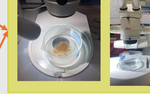
**Stereomicroscope and tweezers** Processed samples by separating microplastics individually from the matrix.
